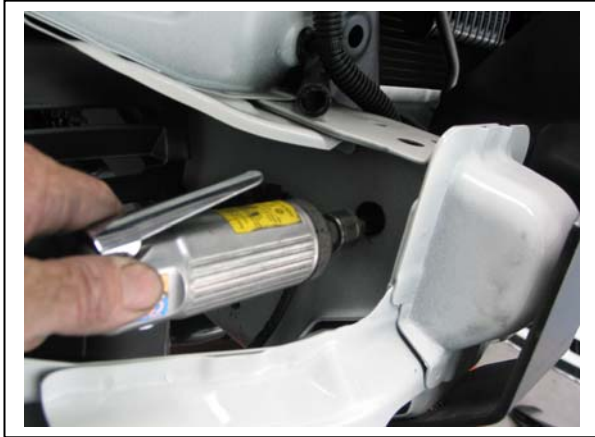
Figure 5 – Enlarging outer chassis hole to 17mm for chassis spacer.
